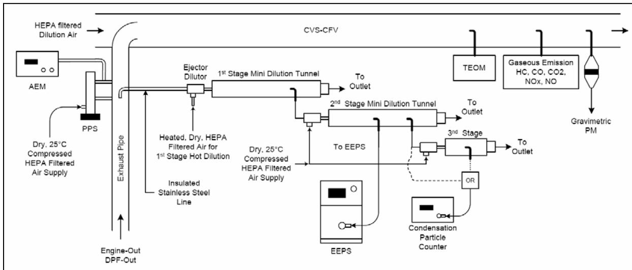
**Figure 1: Measurement Setup**
