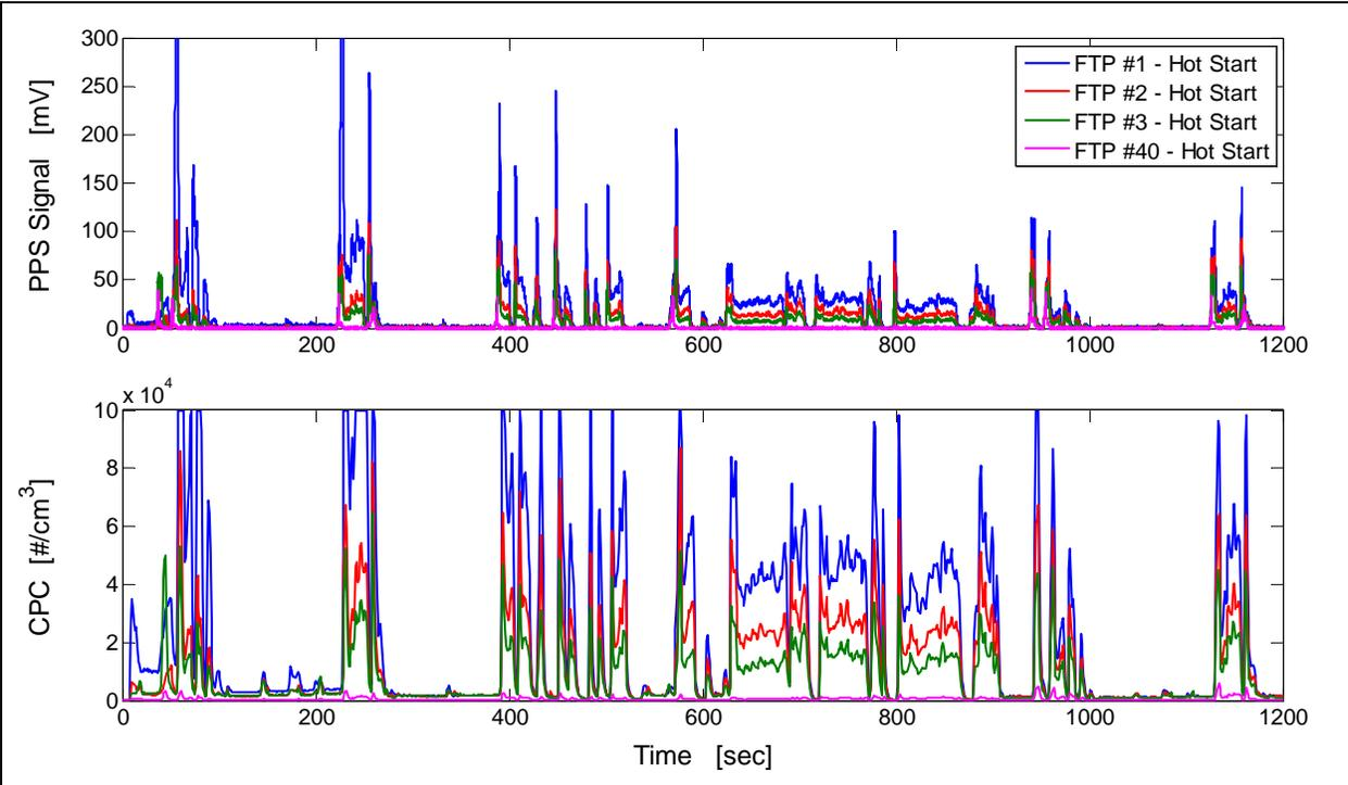
**Figure 3: Comparison of PPS Signal vs. CPC, New DPF (Initial Degreening Phase), CPC Corrected for Dilution (DR = 145)**
