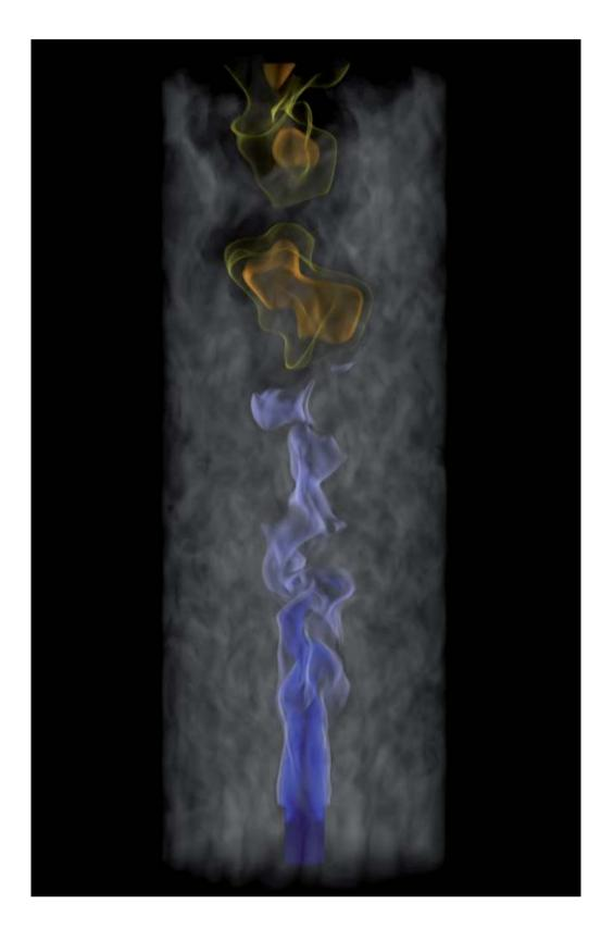
Three dimensional direct numerical simulations are performed to investigate turbulent inhomogeneous autoignition of a laboratoryscale setup where hydrogen is injected into high-temperature, turbulent co-flowing air.
