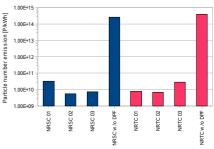
Figure 2. Results of the test cycles with and without particle filter.
