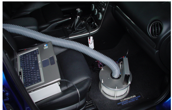
Fig.1: Particle number concentration inside and outside a passenger car (cabin ventilation turned on).
