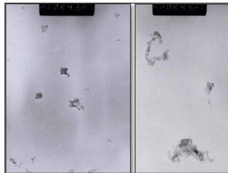
Figure 2. TEM micrograph of diesel particles collected after a DOC.
