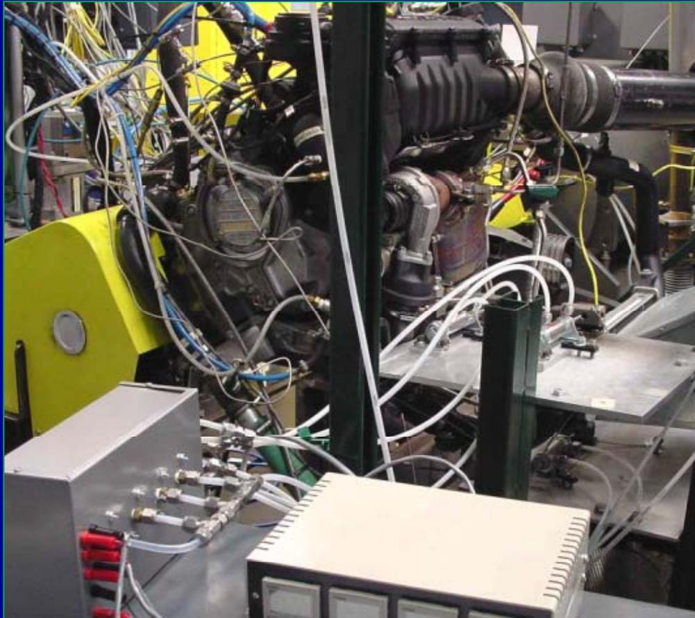
Thermophoretic sampling system installed on a diesel engine
