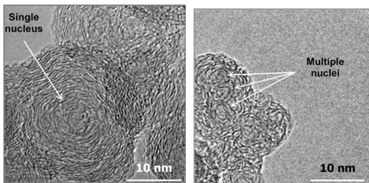
Figure 3. Nanostructures of particles collected from combustion of aromatic-enriched fuel (a) and iso-paraffin-enriched fuel (b), respectively.
