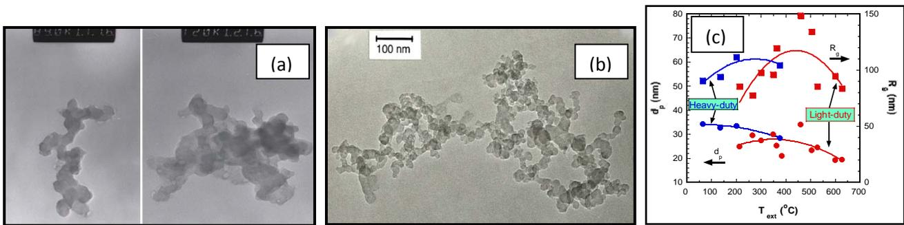
Figure 1. TEM micrographs of diesel particulates collected at idling (a) and 2500 rpm/70% load (b), and particle size distributions as a function of engine operating conditions (c).
