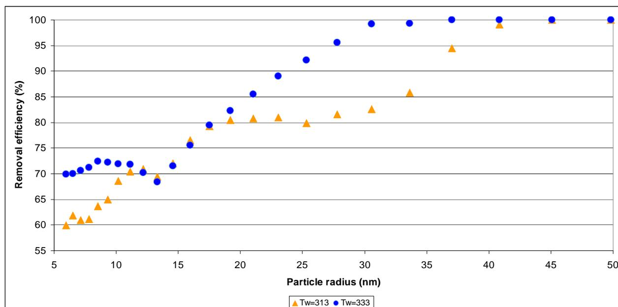
**Fig. 2 – Removal efficiency vs particle radius at two different wall temperatures**
