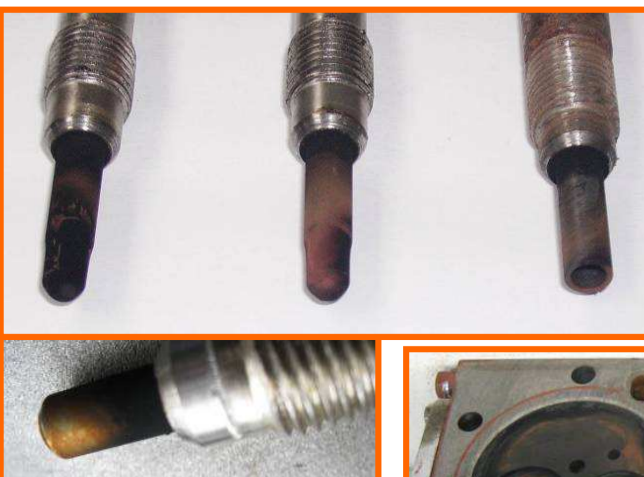
Glow plug after 2 hr at max. load
