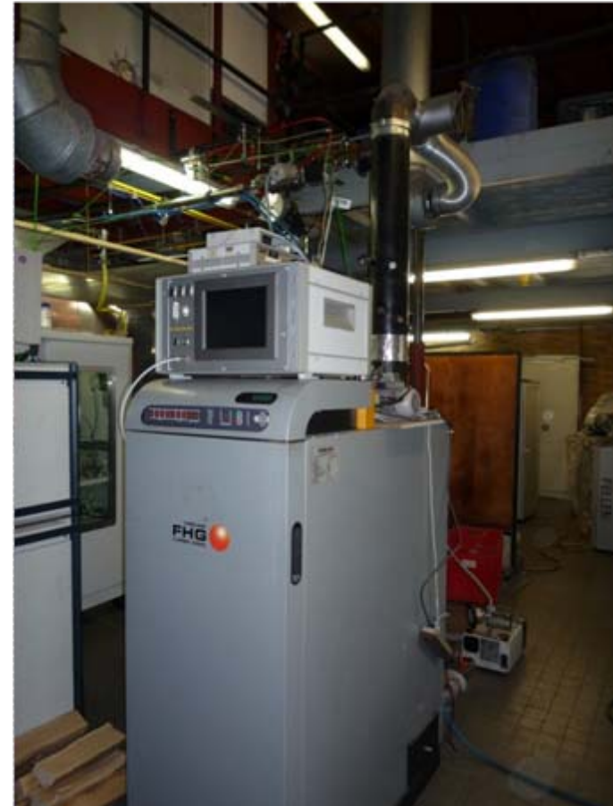
Fröling FHG Turbo 3000 Log wood cauldron (30 kW), automatically fed
