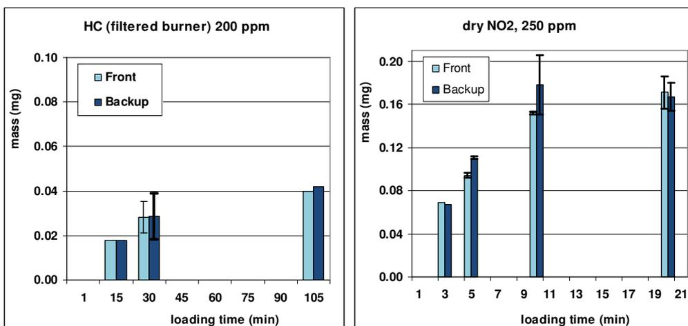
Figure 1: Adsorption of NO<sub>2</sub> and HC on TX40 Filters – Saturation effect
