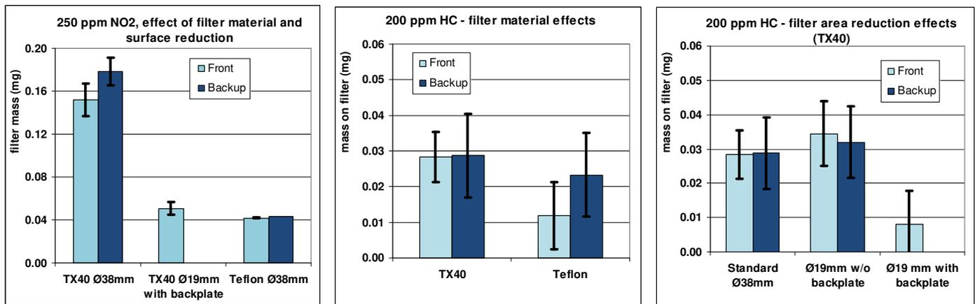
Figure 2: Effect of filter material and filter surface area on adsorption
