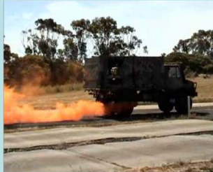
Figure 2. Smoke candle coloured exhaust plume of Unimog truck showing turbulence at rear of vehicle travelling at 20 km/h and plume entry at opening.
