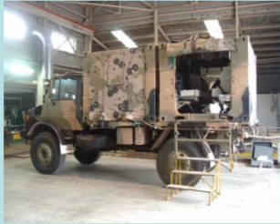
Figure 1. Unimog vehicle with cargo and personnel modules showing the sampling location at the dummy on the passenger side.
