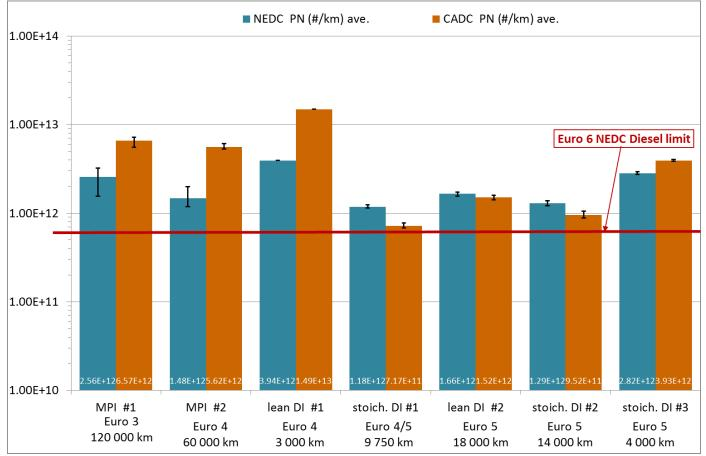
The high particle numbers for the two MPI vehicles (which had similar engines) are believed to be related to engine characteristics rather than the high mileages.
