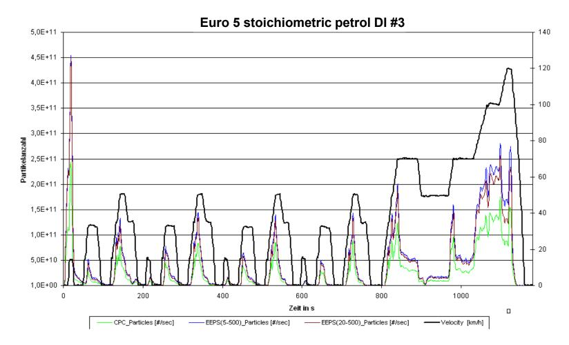
• Note EEPS measures total particles without volatile particle remover
