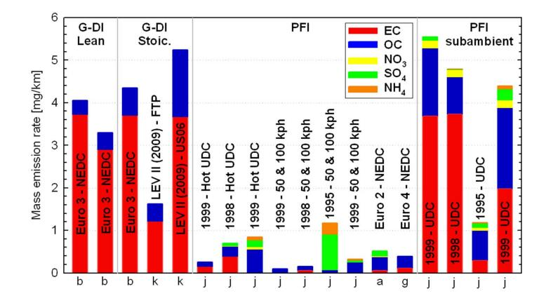
Reported chemical composition of PM emitted from gasoline powered vehicles. The vehicle technology (emission standard or model year) and test cycle are given explicitly on each bar. A: Andersson et al. 2001, b: Mohr et al. 2003,g: Bosteels et al. 2006, j: Schauer et al. 2008, k: Khalek et al. 2010.
