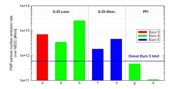
Reported particulate number emissions of gasoline powered vehicles of different fuel injection strategies and emission standards over the NEDC following the legislated procedure for diesel vehicles. d: Andersson et al. 2007, f: Mikulic et al. 2010, g: Bosteels et al. 2006 [ii], h: Braisher et al. 2010 [iii].
