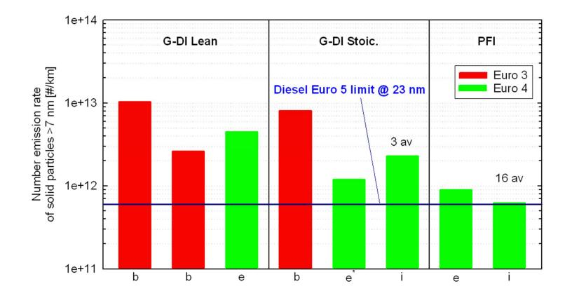
Reported number emission rates of solid particles larger than 7 nm over NEDC for gasoline vehicles of different fuel injection systems and emission standards. b: Mohr et al. 2003, e: Mohr et al. 2006, i: Schreiber et al (2007) [[i]], figures correspond to the average value of 3 stoichiometric G-DI and 16 PFI gasolines, e\*: figure corresponds to the average of 3 tests of a lean G-DI which operated in stoichiometric mode over the particular repetitions.
