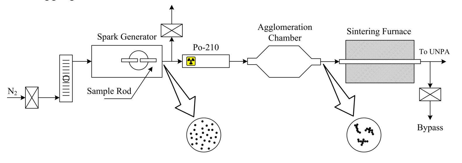
New UNPA measurement device facilitates extended characterization of nanoagglomerates, e.g. primary particle diameter, intrinsic parameters. Measurements for gold, silver and nickel nano-agglomerates genreated from a spark generator are in good agreement with offline-analysis. UNPA can significantly improve the measurement accuracy for loose agglomerates compared to instruments assuming spheres.
