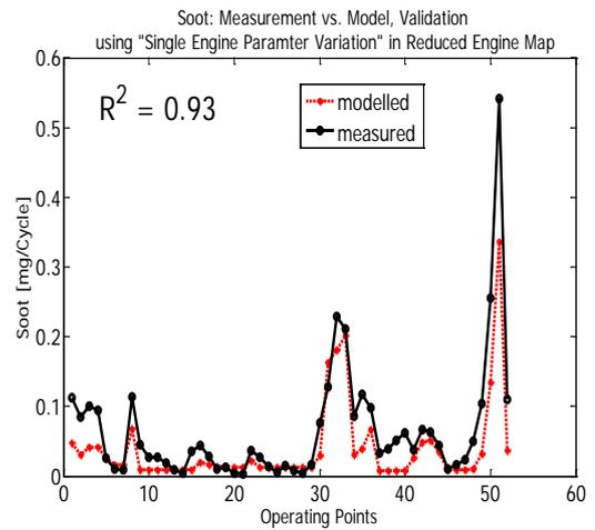
Figure 1: Steady state calibration (left) and validation (right) of the virtual soot sensor.
