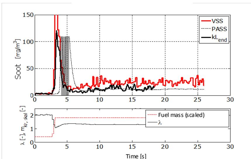
Figure 3: Load transient at 1300 rpm, 2.5 – 12 bar mean effective pressure within 0.5 s.
