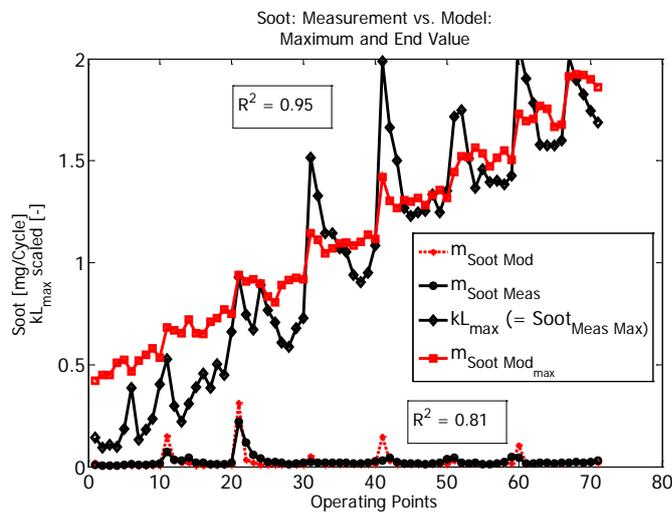
Figure 2: Steady state calibration of the VSS with the maximum modeled soot mass vs. the maximum kL value.
