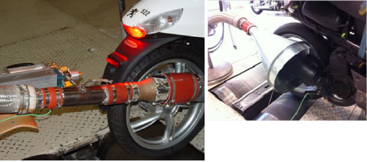
Passage of exhaust gas from tailpipe to CVS: closed (left), open (right)
