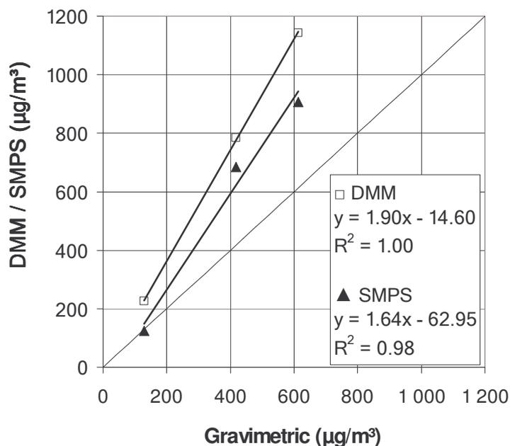
**Figure 1.** Comparison of gravimetric sampling and real-time measuring instruments. The thin line represents the line of equality ( $y = x$ ).
