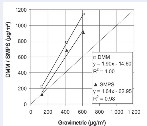
Figure 1. Comparison of gravimetric sampling and real-time measuring instruments DMM and SMPS.
