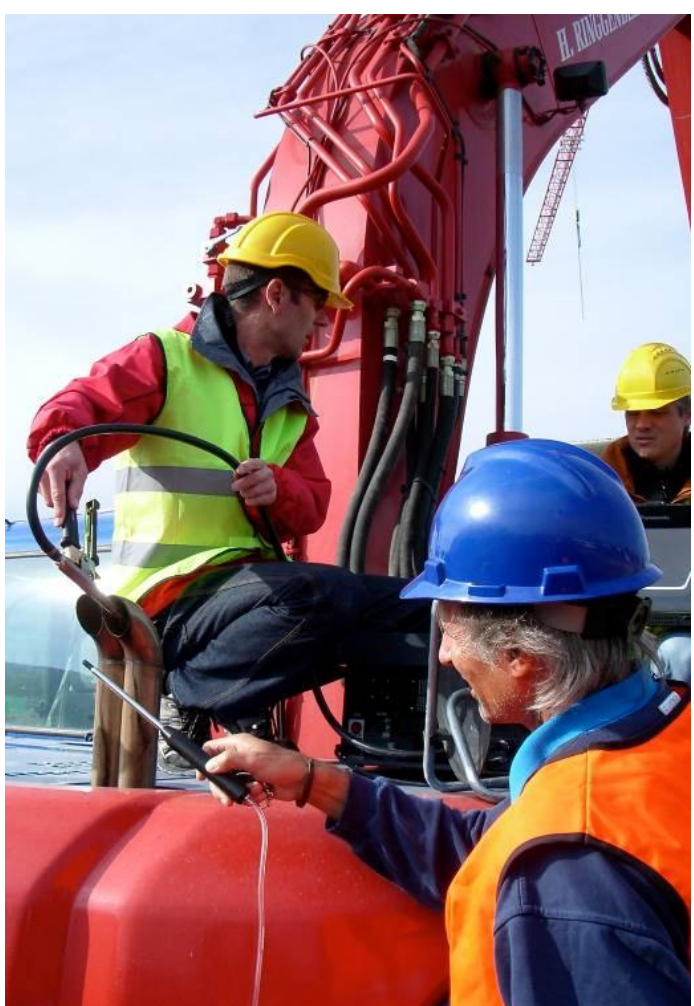
Figure 1: Exhaust measurements on construction machines and seal to declare the control
