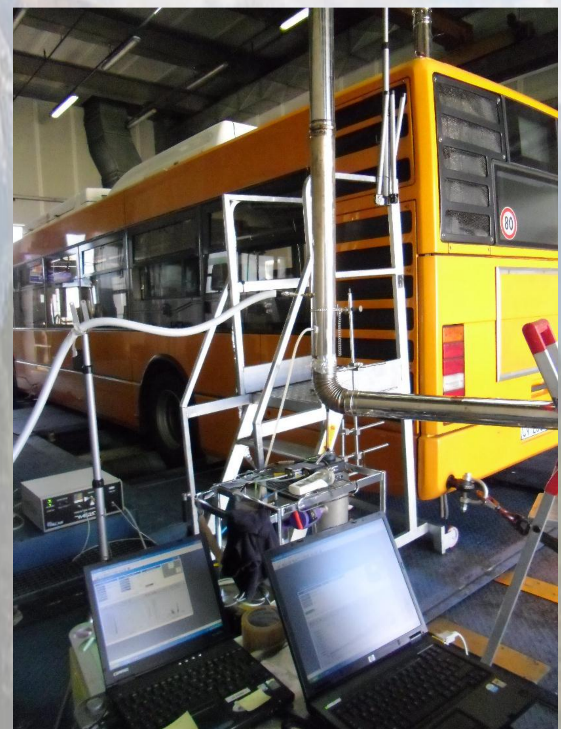
Figure 2 : measurements on the bus on a test bench
