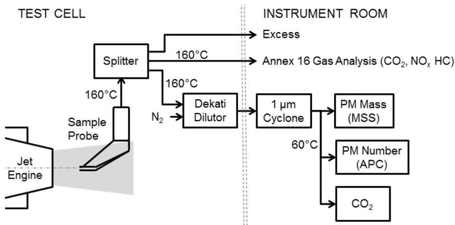
**Figure 1 Simplified schematic of the aircraft gas turbine PM sampling system installed at SR Technics**
