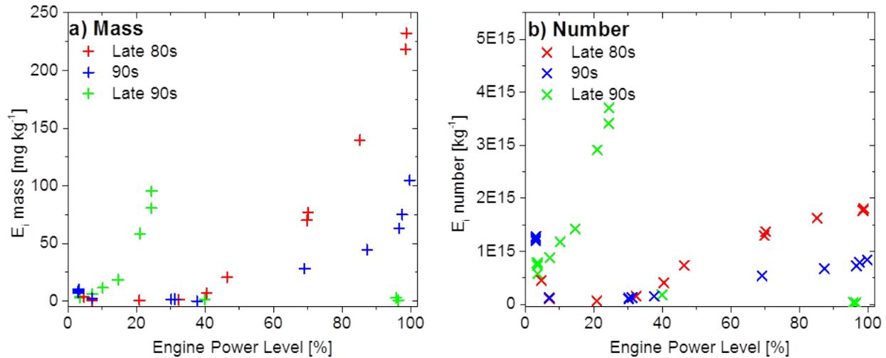
**Figure 2 PM mass emission indices (a) and PM number emission indices (b) for three different engine technologies as a function of engine thrust level**
