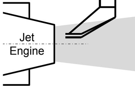
Emissions can have temperatures up to 850°C and velocities near Mach1!
