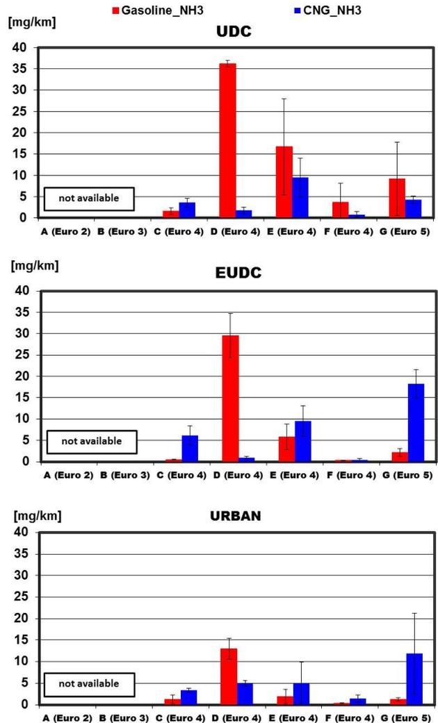
Figure 7 – Ammonia emissions for the fleet vehicles (tests average data with std. dev.)
