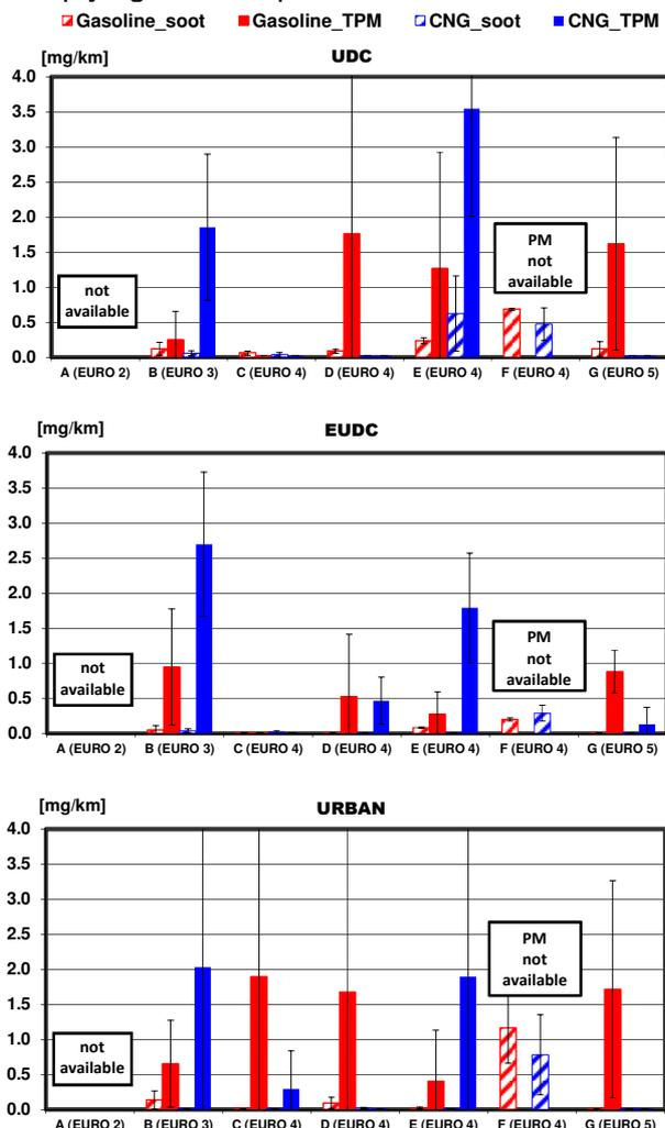
**Figure 2 – TPM vs PM soot emissions for the fleet vehicles (tests average data with std. dev.)**
