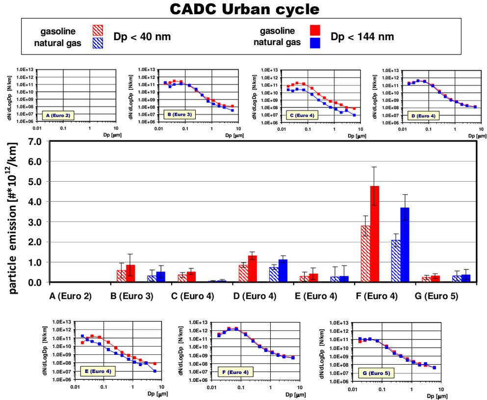
Figure 6 - Nanoparticles and ultrafine particles (Dp< 144 nm) NGVs fleet emissions with each vehicle particle distribution comparing gasoline and NG fuelling - CADC Urban cycle
