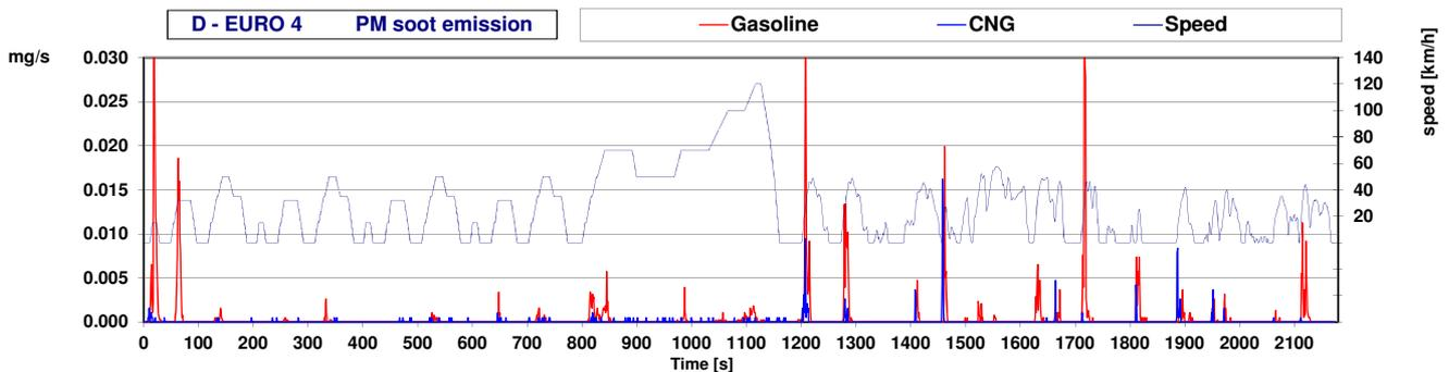
**Figure 3 - Modal PM soot fraction emission - vehicle D (EURO 4)**
