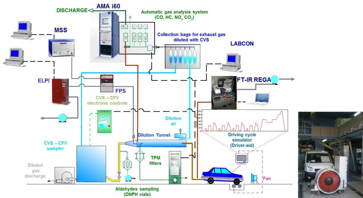
Figure 1 - Exhaust sampling and emissions analysis system
