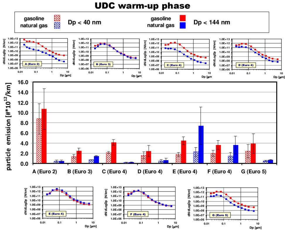
Figure 5 - Nanoparticles and ultrafine particles (Dp< 144 nm) NGVs fleet emissions with each vehicle particle distribution comparing gasoline and NG fuelling - UDC warm up phase
