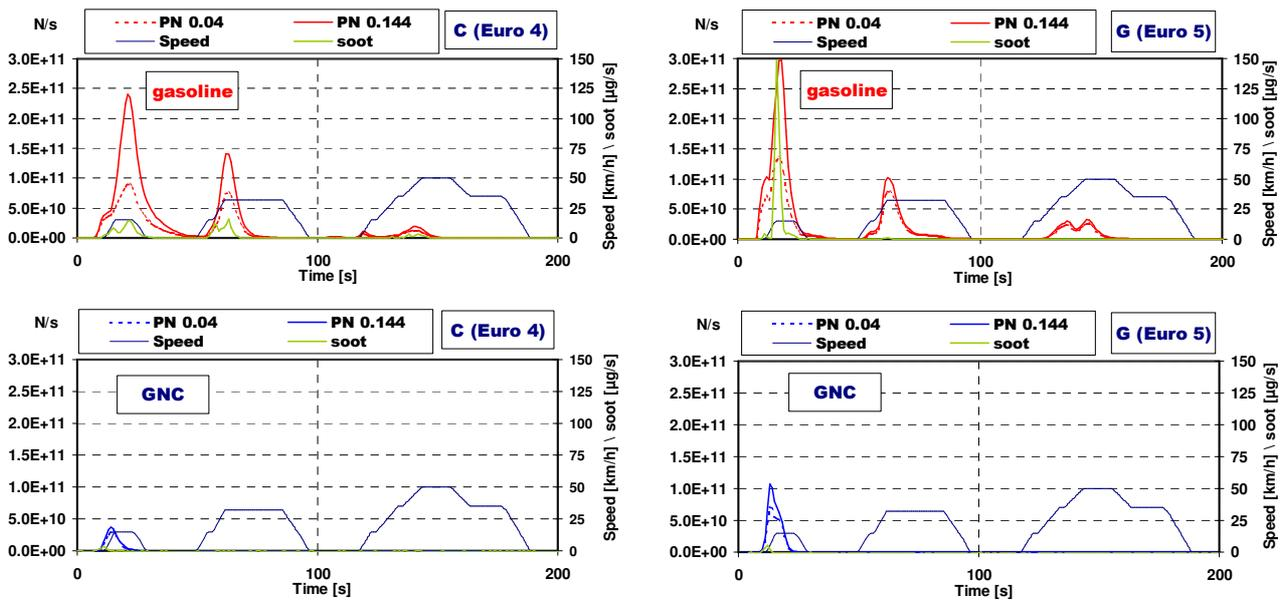
**Figure 4 - Comparison between soot, nanoparticles ( $D_p < 40$  nm) and ultrafine particles ( $D_p < 144$  nm) emissions – UDC warm-up phase (vehicles C and G)**
