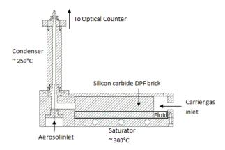
One crucial design criterion was selection of high-temperature working fluids. The short listed candidates including organic oils (DEHS), perfluorocarbons (e.g. Fomblin fluids), silicone fluids (Dow Corning 704, 705 or equivalents) and polyphenylethers (e.g. Santovac 5) were tested experimentally.
