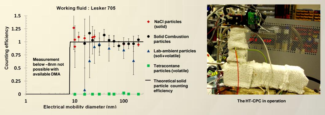
• Without sample pre-heating or dilution, the HT-CPC using DC704 or Lesker705 fluids was able to grow and detect solid particles as predicted by the model.
