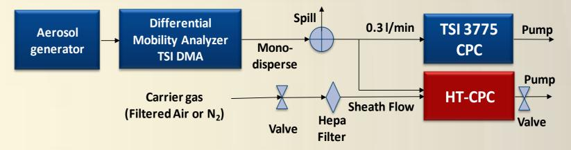
The HT-CPC and TSI CPC were compared and the counting efficiency as a function of particle electrical mobility diameter was obtained.
