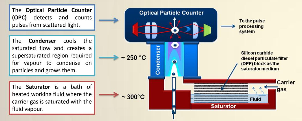
Since the HT-CPC operates at high temperatures, it automatically removes all liquid particles, so that only the stable, solid, ones are measured. This makes the measurement of nanoparticles more reliable.
