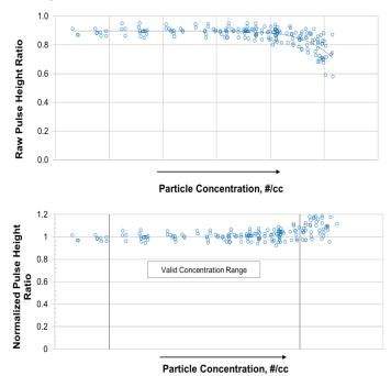
concentrations. The Y Intercept value on this curve is determined individually during calibration to account for instrument to instrument variability.
