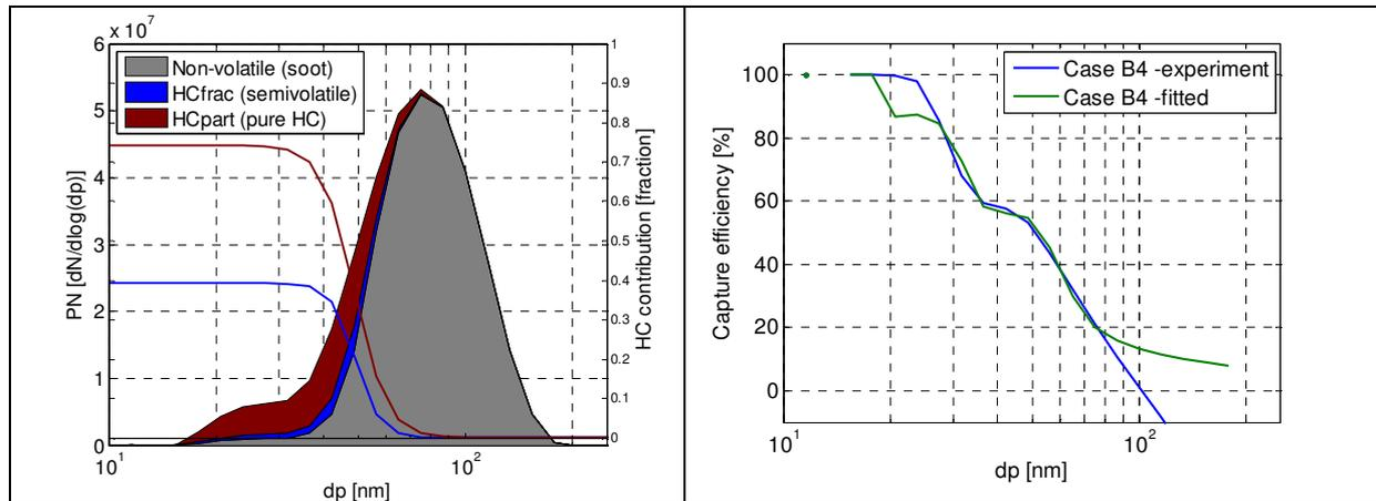
Figure 1. Left: The particle size distribution and the corresponding volatile contribution using a sigmoidal function describing the size-dependent fractions. Right: The experimental and fitted capture efficiencies.
