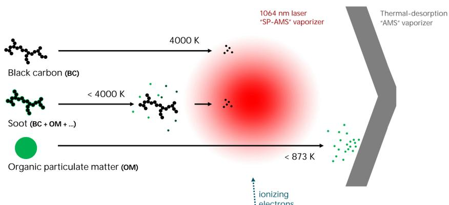
**Fig. 3. SP-AMS particle vaporization.**
