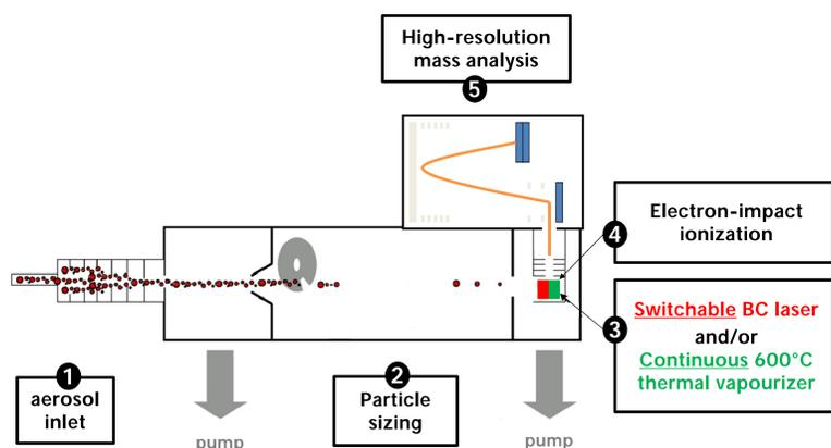
**Fig. 2. The Soot-Particle Aerosol Mass Spectrometer (SP-AMS).**
