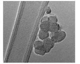
Solvent extraction and centrifugation have been used to prepare suitable samples for TEM analysis onto graphene oxide TEM support films.
