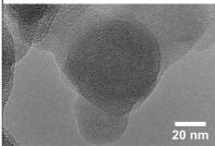
Exhaust primary particles were found in the range 20-70nm, with a mean diameter of 38.6nm. Only 1.2% were smaller than 30nm. Exhaust soot exhibits a nearly amorphous nanostructure.
