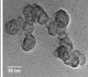
Soot agglomerates have a modest branched morphology, and exist in clusters and chainlike structures in a range from 40 to 400nm. Agglomerates show an average length of 150nm and are composed of spherical primary particles of 18-60nm.
