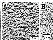
Differences in nanostructure may reflect a combination of different operating conditions, combustion temperatures and chemical species contributing to particle growth at various stages.
