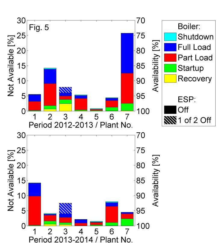
Fig. 5 allocates phases with unavailable ESP to boiler operating modes.
