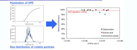
Volatile particle removal performance can be improved by the reduced VPR penetration .... Removal efficiencies were corrected by VPR penetration and size distribution of
