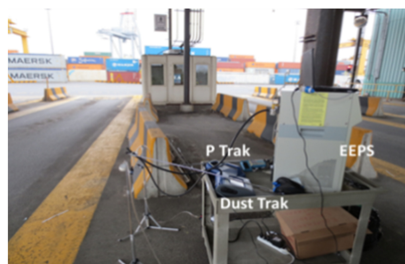
Figure 2: Stationary measurements at the terminal
