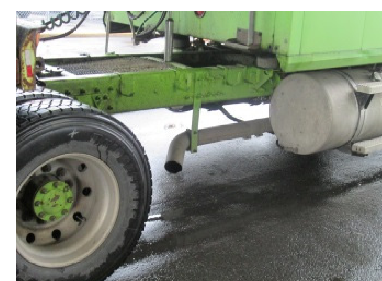
Figure 4: Older truck with exhaust pipe at the level of the workers
