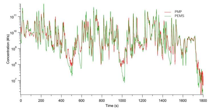
Unavoidable time misalignment due to **different response time** of the systems and **time delay** between tailpipe and CVS: Reported results are cycle average emission factor **#/km**
