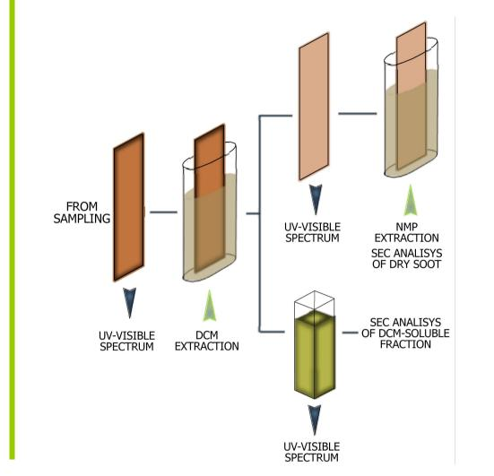
L-PAH adsorbed on the deposited carbon particulate matter were separated from the solid carbon (dry soot) by solubilization in Dichloromethane (DCM) and recovered for spectroscopic (UV-visible) the and chromatographic (SEC) characterization. The UV-visible spectrum in the 190–250 nm wavelength range of the L-PAH were obtained by difference between the spectra measured on the quartz plate before and after the DCM extraction.
