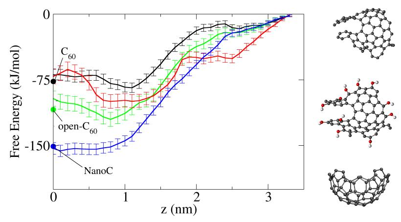
Open-C60 binding depth 120 kJ/mol, 1.4 larger than C60 and 0.8 less than nanoC Nano-OH great binding at lipid/water
