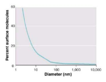
%molecules on surface to the total molecules increases exponentially when diameter decreases in range 1-100nm. (Oberdorster, 2005)
