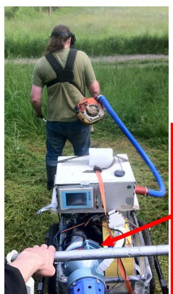
30-60 m<sup>3</sup>/min sampling on **142/150 mm filters** for analyses (i.e. PAH) and toxicological assays
