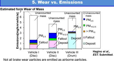
airborne PM<sub>2.5</sub> : 8% (vehicle I), 21% (vehicle II), 2% (vehicle III)
