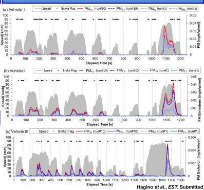
The brake wear particles can be released by brake abrasion and the swirling airflow resulting from the rotor or drum after prior braking events.
