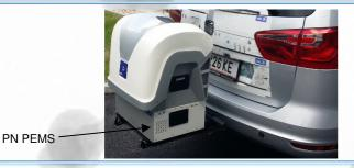
Figure 1: Installation of the AVL PN and Gas PEMS iS on the trailer hook of a passenger car.
