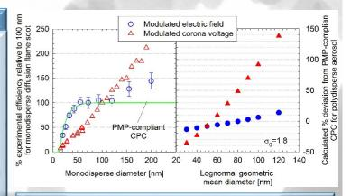
Figure 2: Left-hand panel: Experimentally determined size dependence on monodisperse soot particles for the original particle detector (modulated corona voltage) and a prototype one (modulated electric field) developed for the PN-PEMS. Right-hand panel: Calculated correlation of the two sensors against the a PMP-compliant CPC for polydisperse lognormal distributions (geometric standard deviation of 1.8).
