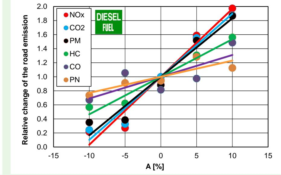
Relative change of the road emission of pollution with the change of the route grade for vehicles fitted with gasoline and Diesel engine
