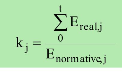
**j** – exhaust component, for which the emission indicator was determined **E**<sub>real,i</sub> – on-road emission under real traffic from the start of the test [g/km] Enormative, j – normative on-road emission according to Euro 5 [g/km]
