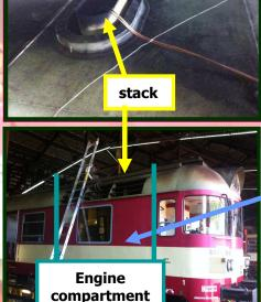
Severe environment: 0-55°C, vibrations, "rail dust" (a mixture of soot, oil, grease, iron oxide brake dust), lack of access during most of the train run
