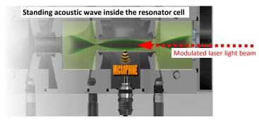
A standing acoustic wave in the resonator is generated by stimulating the particles with a modulated light source.
