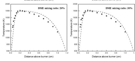
Peak flame temperature as a function of DME mixing ratio
