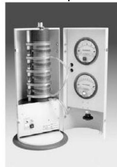
Particles collected on the two last stages of the impactor ( $d_{50} = 100$  nm and  $d_{50} = 56$  nm) considered for analyses
