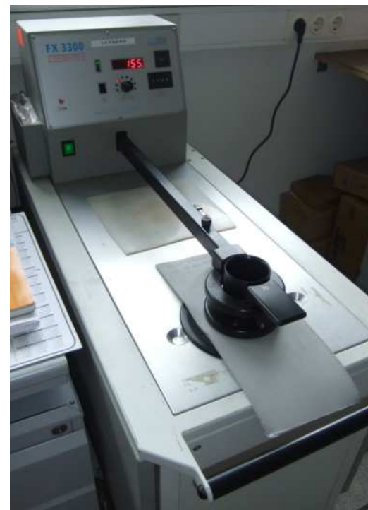
Testing machine for permeability
