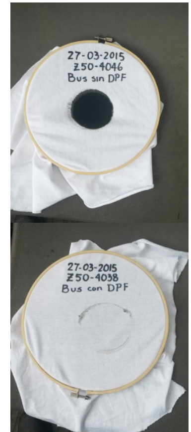
Visual indicator of PM emission in Transmilenio buses with and without DPF – 2015.
