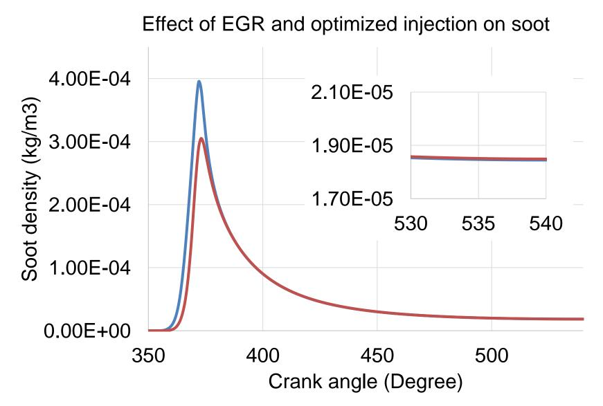
Increasing EGR rate  $\rightarrow$  Lowering cylinder oxygen content  $\rightarrow$ Increasing exhaust soot
