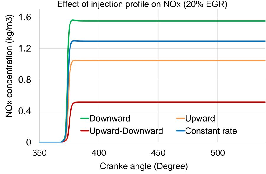
Upward-Downward profile generates the lowest NOx concentration at the same EGR rate
