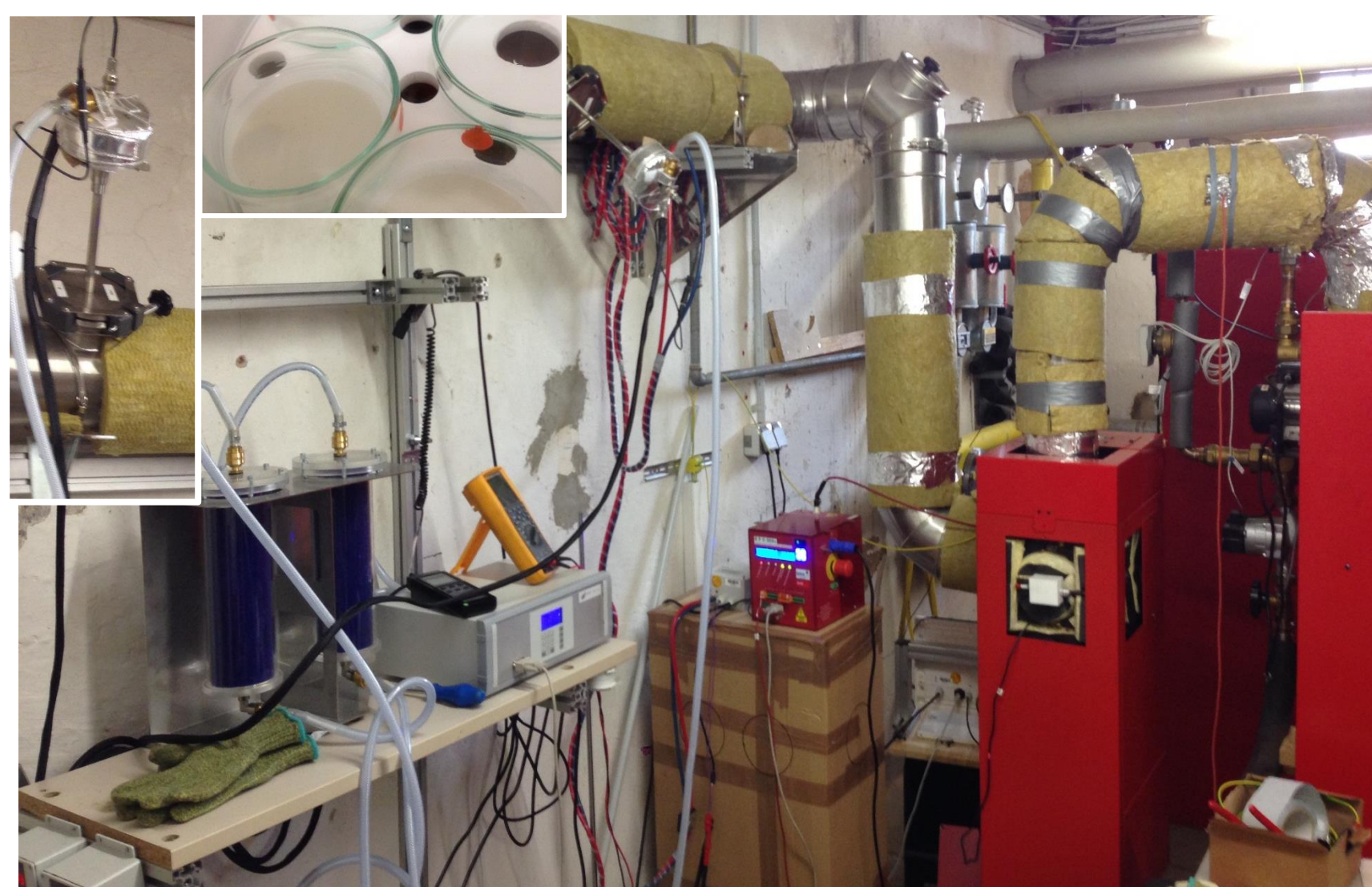
Figure 1: Used test system, electrostatic precipitator and 50 kW th logwood boiler; Upper left: Used VDI 2066 probe for sampling (EDX, REM)
