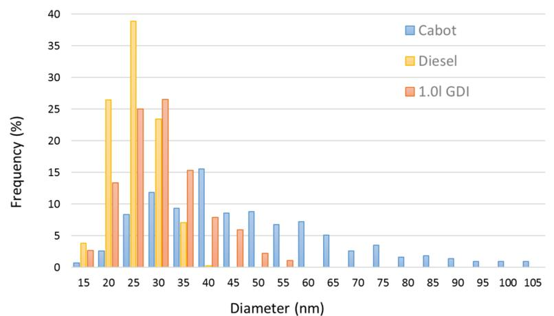
Figure 4. Primary particle size comparison between carbon black (Cabot), diesel and 1.0l GDI soot.
