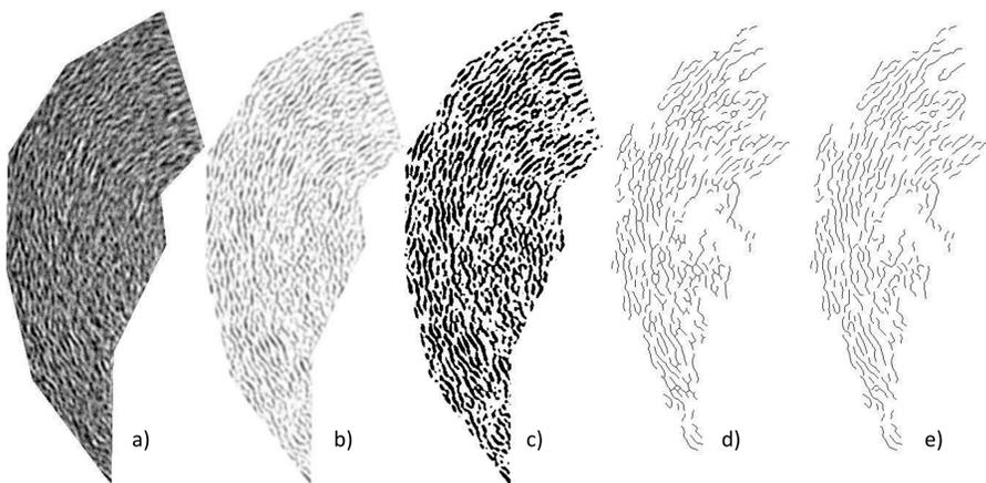
Figure 1. Inverted image at various stages of processing. a) Original HRTEM image. b) After contrast enhancement, Gaussian blur and white top hat transformation. c) After binarization. d) After skeletonization with border fringes and artefacts removed. e) Final image after fringe cleaning algorithm.
