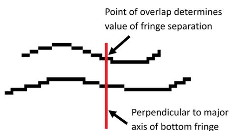
Figure 3. Representation of fringe separation measurement method.
