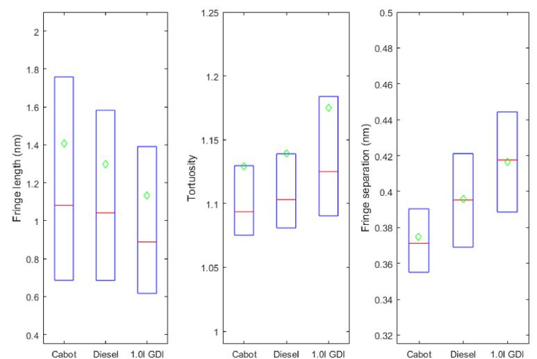
Figure 5. Comparison of nanostructure parameters between the three types of soot. Green marks indicate the mean value, red the median and blue the interquartile range.
