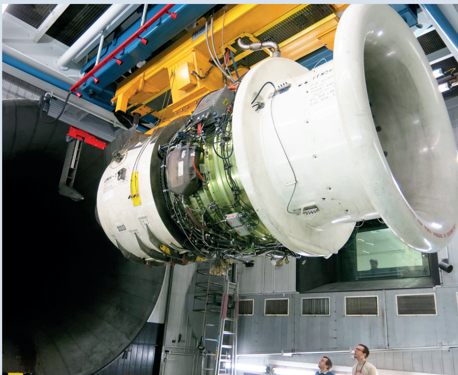
Engine in the test cell of SR Technics with the exhaust sampling probe at the engine exhaust exit plane (left)
