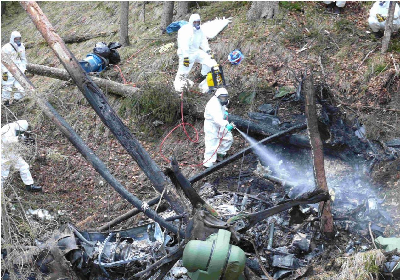
*Application of fiber binder on helicopter wreck*
