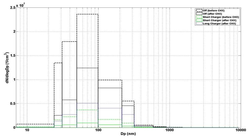
→ By optimising the charger–CHX geometry we are reaching 96% removal efficiency
