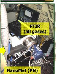
Lack of space: Confinement into "dead-end isle" of engine compartment (nothing can be put outside of the train, no opening to conductor cabin, one isle to remain free for train engineer to walk through during turnarounds).
