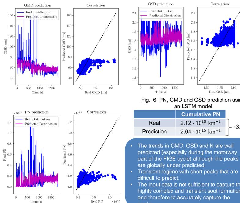
Fig. 6: PN, GMD and GSD prediction using an LSTM model
