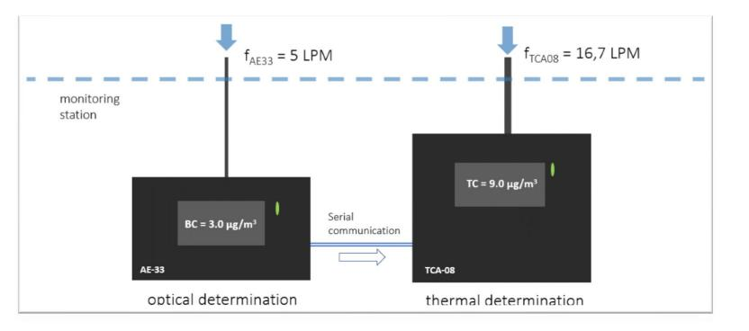
thermal analysis. While one channel is collecting its sample for the next time-base period, the other channel is analyzing the sample collected during the previous period.
